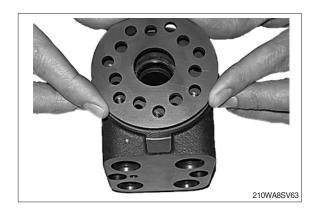
(25) Guide the cardan shaft (13) down into the bore so that the slot is parallel with the connection flange ports and lines up with the cross pin (11).
