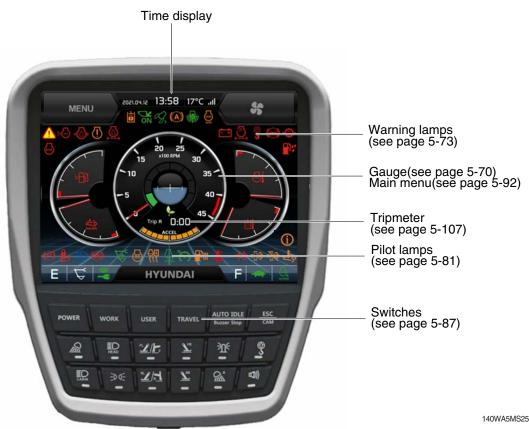
\* The warning lamp pops up and/or blinks and the buzzer sounds when the machine has a problem.
