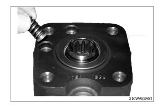
(42) Place O-rings (40) on adjusting screws (25).
