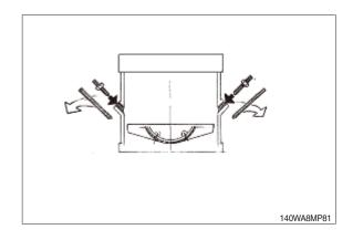
▲ Assemble pump support plate.
