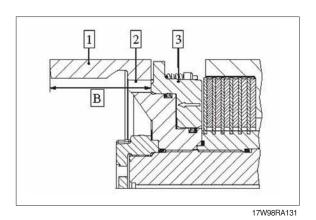
(30) Secure slotted nut with cylindrical screw (see also figure RA127).
