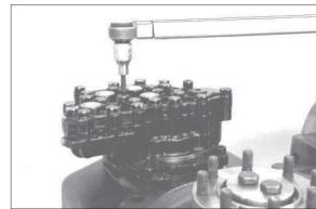
27) Install both screw-in sleeves and screw plug (see arrow) with O-rings.
