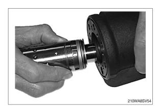
(16) The spool set will push out the assembly tool guide. The shaft seal (5) is now installed.
