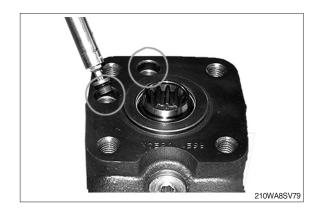
(40) Place one ball (27) in each of the shock valve cavities.
