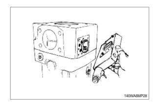
(3) Remove O-ring, measuring piston with bushing and spring.
