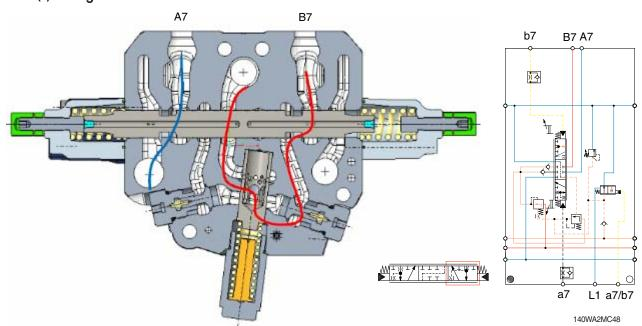
When the pilot pressure is led to the port b7, the oil from the pump flows to the port B7 and oil from the motor flows into the tank through the port A7.
