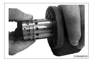
(25) Take the ring (10), bearing races and needle bearing (7) from the spool and sleeve set (2).
