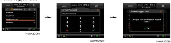
• The logged faults of the MCU, engine ECM, FATC, AAVM (option) can be deleted by this menu.
