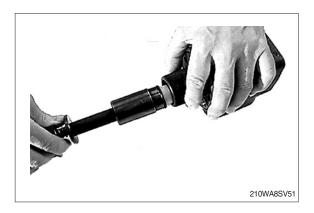
(13) Press and turn the shaft seal (5) into position in the housing.
