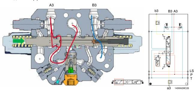
When the pilot pressure is led to the port a3, the oil from the pump flows to the cylinder port A3 and oil from the cylinder flows into the tank through the cylinder port B3.
