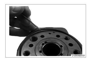
(23) Shake out the check valve ball (3), suction valve pins (34), balls (33) and ball (36).
