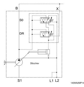
The pressure controller limits the maximum pressure at the pump outlet within the control range of the variable pump. The variable pump only supplies as much hy-draulic fluid as is required by the consumers. If the operating pressure exceeds the pressure setting at the pressure valve, the valve opens the connection from P-chan-nel (high pressure) to A-channel (stroking pressure) and the pump will regulate to a smaller displacement to reduce the control differential.
