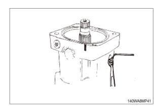
(6) Remove joint pin for swivel cradle.
