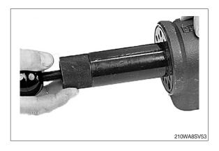
(15) With a light turning movement, guide the spool and sleeve into the bore.Fit the spool set holding the cross pin (11) horizontal.
