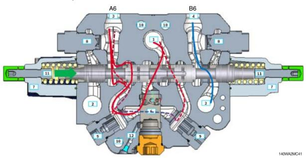
When the pilot pressure is led to the port a6, the oil from the pump flows to the port A6 and oil from the motor flows into the tank through the port B6.
