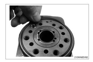
(24) Place the distributor plate (16) so that the channel holes match the holes in the housing.
