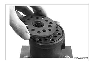
(20) Remove the threaded bushing/ball stop (4) from housing.
