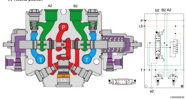
The spool is in neutral position, pump is in low pressure stand-by. The A2 and B2 ports are not connected to the pumps nor the tank.
