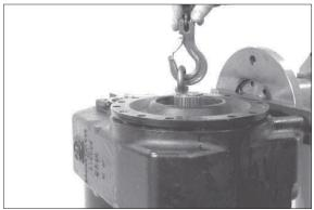
20) Press output gear out of ball bearing/cover - remove releasing oil screen sheet.
