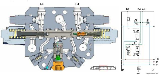
Neutral position of arm spool, all connections of the spool are closed and the A4 and B4 ports are not connected to the pump nor tank.
