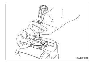
(4) Loosen lock nut (14-6) and adjusting nut (12) with spanners on them respectively, and take out handle section as one body.
