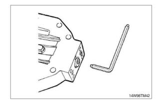
(2) Remove piston with piston ring.
