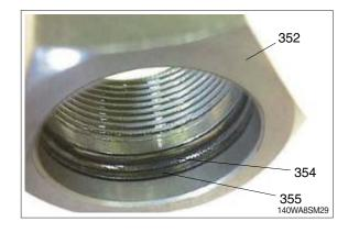
④ Grease and install the O-ring (353) in the nut spot facing (352).
