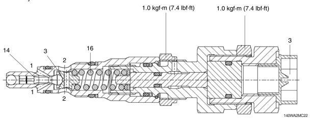
\* For the case of unintentional adjustment during assembly process, we would recommend to mark the positions by sealing wax.
