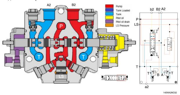
When the pilot pressure is led to the port b2, the oil from the pump flows to the cylinder port B2 and oil from the cylinder flows into the tank through the cylinder port A2.
