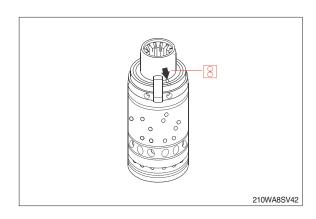
(4) Guide the spool into the sleeve (2). If the spool and sleeve has marks as shown above, these must be placed on same side. Make sure the centering springs (12) are placed into the slot.
