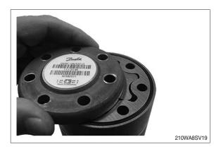
(11) Lift the gearwheel set (17a) off the unit. Remove the two O-rings (18).
