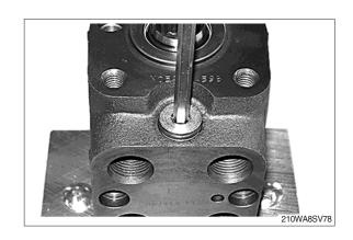
(39) Place O-ring (41) on the shock valve seats (28). Screw in the seats (28) with a 2.75 mm allan key into the cavities indicated by the circles.
