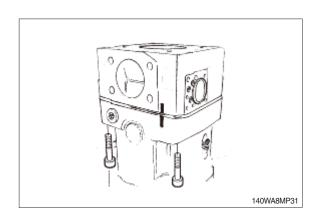
(6) Remove port plate with control plate. Disassemble regulator.
