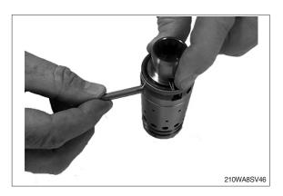
(8) Fit bearing races and needle bearing (7) as shown on the next drawing.
