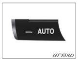
① Auto air conditioner and heater system automatically keeps the optimum condition in accordance with operator's temperature configuration sensing ambient and cabin inside temperature.
