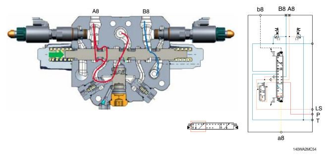
When the pilot pressure is led to the port a8, the oil from the pump flows to the port A8 and oil from the cylinder flows into the tank through the port B8.
