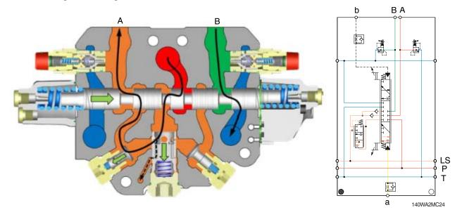
Pilot pressure on A-side opens the spool and connects pump to consumer A.
