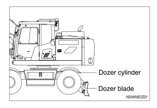
② Disconnect dozer cylinder hoses (1), and put plugs on cylinder pipe.
