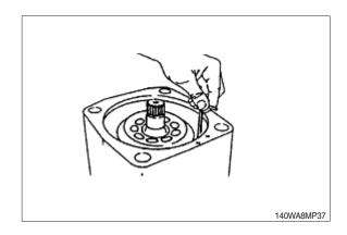
(2) Remove retaining segments with screws.
