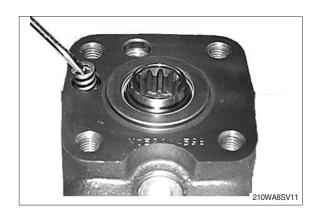
(3) Remove the balls for shock valves (27).
