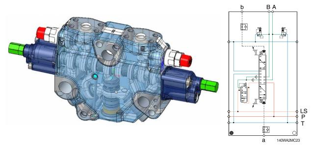
In neutral position, no connection between pump an consumer and also no connection between consumer an tank channel.
