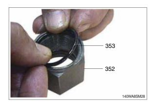
⑤ Install and tighten the nut (352) to the required torque.
