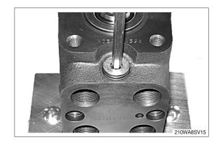
(7) Remove the spring for relief valve (31).
