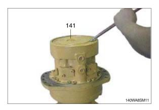
(4) Tighten the screw in the piston and tighten the nut until the motor shaft turns freely.
