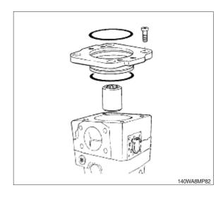
(22) Install measuring piston with O-rings.
