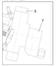
5 Hydraulic stroke limiter7 Motion control valve assy
