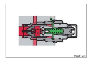
(3) Remove counter-balance valve. Inspect O-ring
