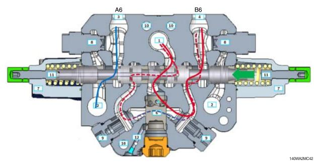
When the pilot pressure is led to the port b6, the oil from the pump flows to the port B6 and oil from the motor flows into the tank through the port A6.
