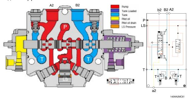
When the pilot pressure is led to the port a2, the oil from the pump flows to the cylinder port A2 and oil from the cylinder flows into the tank through cylinder port B2.
