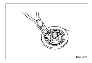
(2) Screw in sheet metal screw into the holes fitted with rubber.Pull out seal with pliers.
