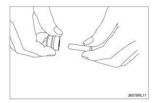
(13) Remove O-ring (8-3) and seal (6-4) from plug (6-1).
