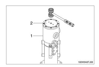
(4) Fit shim (5), and spacer (4) to hub (1) of turning joint upside.
