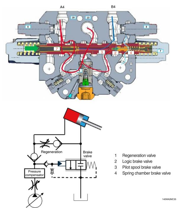
Pump flow is connected over compensator and load holding valve to the port A4.
