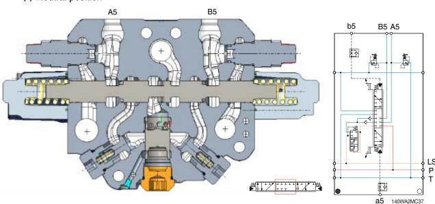
Neutral position of bucket spool, all connections of the spool are closed and the A5 and B5 ports are not connected to the pump nor tank.
