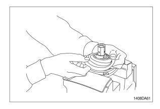
(6) Loosen adjusting nut (12) and swash plate (11) with spanners on them respectively, and remove them.
