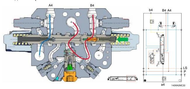
When the pilot pressure is led to the port b4 the oil from the pump flows to the cylinder port B4 and oil from the cylinder flows into the tank through the cylinder port A4.
