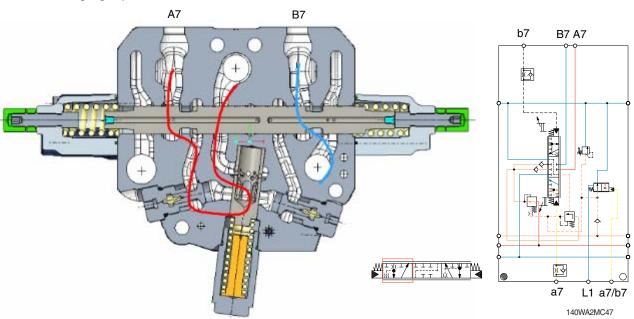
When the pilot pressure is led to the port a7, the oil from the pump flows to the port A7 and oil from the motor flows into the tank through the port B7.
