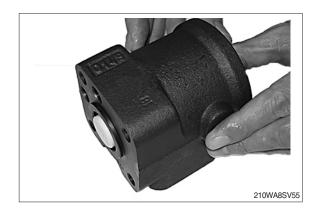
(17) Place the steering unit housing on the holding tool on the steering column end.Put the check valve ball (3) into the hole indicated by the circle.
