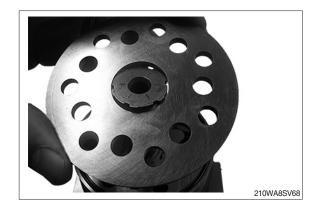
(30) Place the 2 O-rings (18) in the two groves in the valve housing assembly (54). Place the valve housing assembly so that the one and only M8 thread whole points upwards and direction port face. Make sure that channel holes match the holes in the distributor plate (16).
