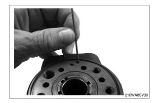
(22) Remove the O-ring (18) from housing.
