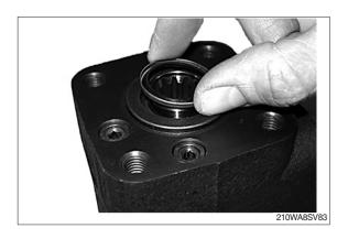
(44) Fit the dust seal ring in the housing using special tool for dust seal assembly and a plastic hammer.
