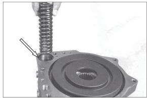
62) Oil O-ring and insert it into annular groove of input housing.
