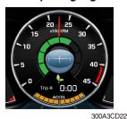
① This displays the engine speed.
