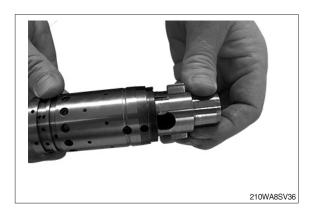
(28) Press the neutral position springs (12) out of the slot of the spool.
