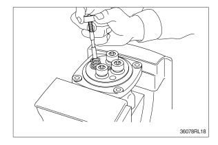
(3) Assemble O-ring (8-3) onto plug (6-1).
