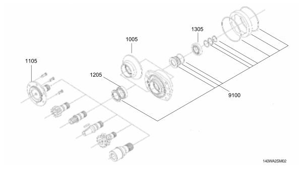
1005 Bearing housing1105 Pinion shaft
