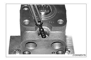
(37) Install the spring (31) on top of the piston (32).
