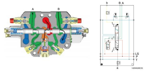
Pilot pressure on A-side opens the spool and connects pump to consumer A.
