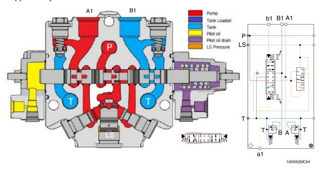
When the pilot pressure is led to the port a1, the oil from the pump flows to the cylinder port A1 and oil from the cylinder flows into the tank through cylinder port B1.
