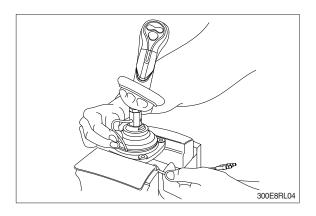
(16) Determine handle direction, tighten lock nut (14-6) to specified torque to fix handle.
