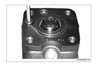
(2) Remove the springs with trust pads for shock valves (26).
