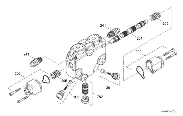
201Spool assy205Spring361Spool assy202Cover assy241Pressure relief valve782Spool assy
