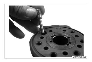
(21) Remove the ball stop (35) from housing.
