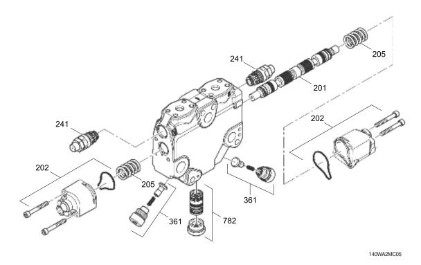
201Spool assy205Spring361Spool assy202Cover assy241Pressure relief valve782Spool assy
