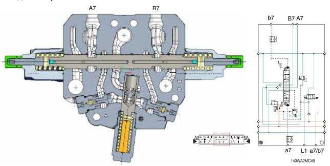
Neutral position of swing spool, all connections of the spool are closed and the A7 and B7 ports are not connected to the pump nor tank.
