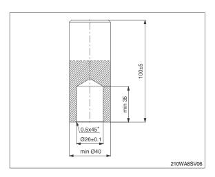
(3) Assembly tool for shaft seal, O-ring.
