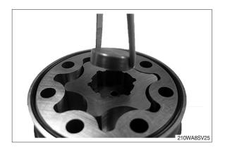
(17) Lift the gearwheel set (17) off the unit. Remove the two O-rings (18).
