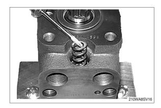
(8) Remove the piston for relief valve (32).
