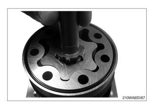
(29) Place the middle distributor plate (16) so that the channel holes match the holes in the gear set.
