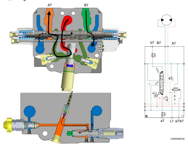
Pilot signal on port A7 opens pump -> port A7 and also port B7 -> tank channel.
