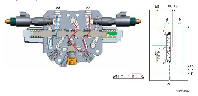
When the pilot pressure is led to the port b8, the oil from the pump flows to the port B8 and oil from the cylinder flows into the tank through the port A8.
