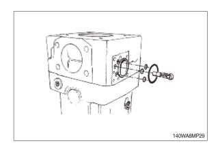
(4) Remove pump support plate.
