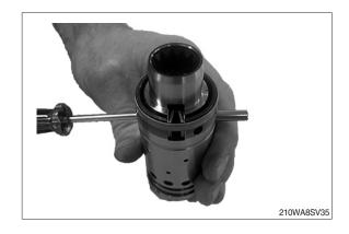
(27) Carefully press the spool out of the sleeve.
