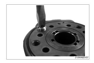
(19) Put the check valve ball (36) into the hole indicated by the circle.Ball (36) is only present in OSPD LS with check valve in LS line.
