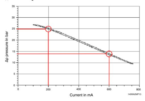
Because the LS controller can be overridden with a solenoid. It need the following two pieces of information for the setting point. Current and  $\Delta p$  pressure. You can get this information individually from your HD Hyundai Construction Equipment dealer.
