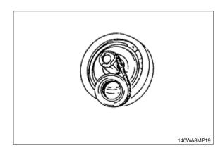
(2) Loosen retaining ring and remove it, press away front cover.
