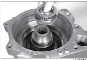
20) Remove pressure piece and compression spring.
