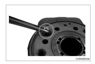
(18) Screw the threaded bushing/ball stop (4) lightly into the check valve bore. The top of the bush must lie just below the surface of the housing.
