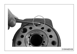
(20) Screw the ball stop (35) into the LS check valve bore.
