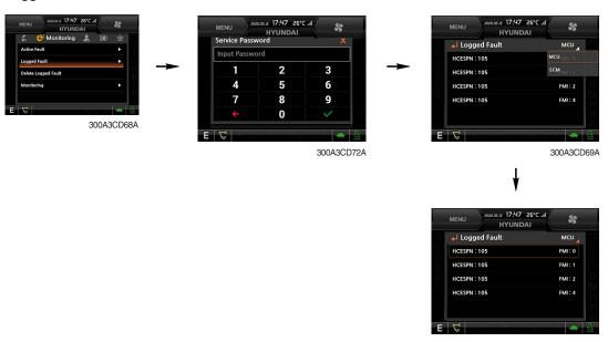
· The logged faults of the MCU, ECM, FATC, AAVM (option) can be checked by this menu.
