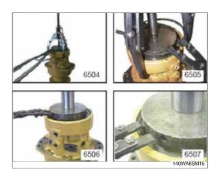
Install a new O-ring (143) coated with anti-oxidizing grease in the groove of brake body (101).
