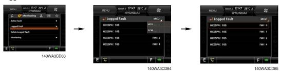
• The logged faults of the MCU, engine ECM, FATC, AAVM (option) can be checked by this menu.
