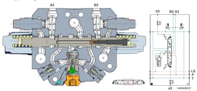
Neutral position of boom spool, port A3 is connected to tank by a small notch. All other connections of the spool are closed.
