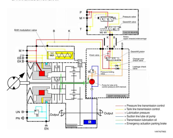
Measuring points-Transmission/Shift interlock :
