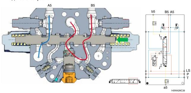
When the pilot pressure is led to the port b5, the oil from the pump flows to the cylinder port B5 and oil from the cylinder flows into the tank through the cylinder port A5.
