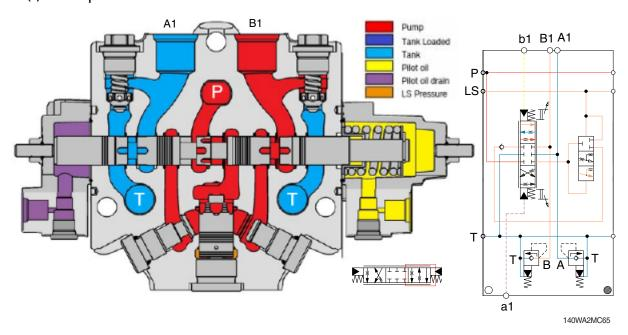
When the pilot pressure is led to B1 side, the oil from the pump flows to the cylinder port B1 and oil from the cylinder flows into the tank through the cylinder port A1.
