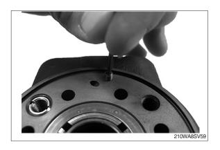
(21) Place a ball (33) in the two bolt holes indicated by the circles.
