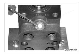
(6) Screw out the adjusting screw for relief valve (30).
