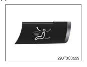
① Operating this switch, it beeps and displays symbol of each mode in the following order. (Face → Face/Rear → Face/Rear/Foot → Foot → Def/Foot)
