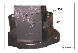
⑤ Remove the block (300) and discard the O-rings (308). (See spare parts).
