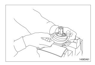
(13) Fit boot (14-1) and lock nut (14-6), and handle subassembly is assembled completely.
