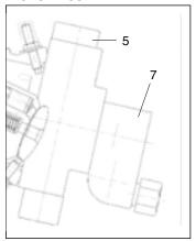
5 Hydraulic stroke limiter 7 Motion control valve assy
