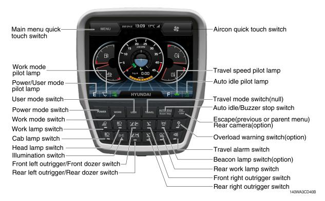
When some of the switches are selected, the pilot lamps are displayed on the LCD. Refer to page 5-81 for details.
