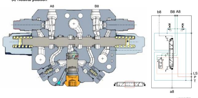
Neutral position of option spool, all connections of the spool are closed and the A8 and B8 ports are not connected to the pump nor tank.
