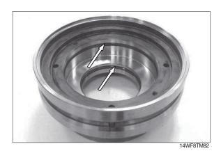
19) Remove axial roller cage with both thrust washers.
