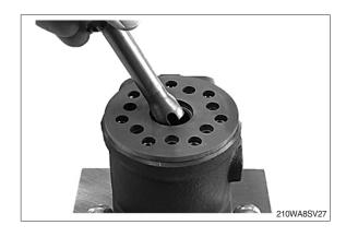
(19) Remove the distributor plate (16) from the housing.
