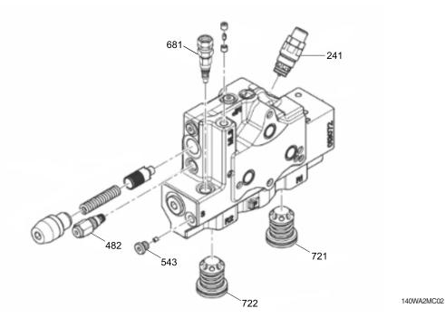
241 Pressure relief valve482 Flow valve
