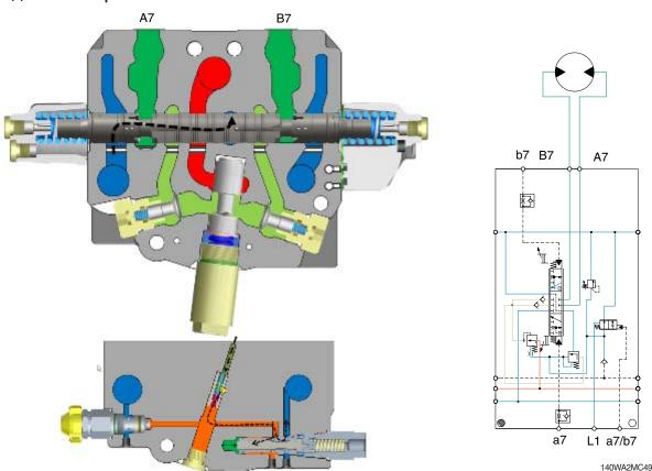
The pump channel is always connected to the compensator. If pump pressure is higher than LS + spring setting of the LS-compensator, the LS compensator will be closed.
