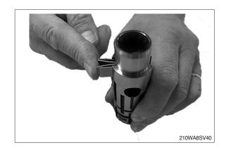
(2) Configuration of spring set (12). There can be different numbers of curved springs depending on configuration of spring set. There can be 2, 4 or 6 curved
