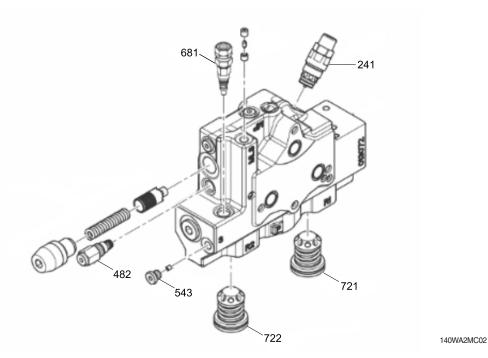
241 Pressure relief valve482 Flow valve
