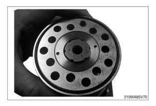
(31) Place the rear distributor plate (16) so that the channel holes match the holes in valve housing assembly (54).
