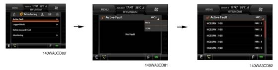
· The active faults of the MCU, engine ECM, FATC, AAVM (option) can be checked by this menu.
