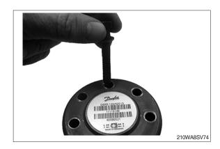
(35) Fit the six screws (23) with new washers (20) and insert them. In case the unit has pin bolt screw, this must be inserted where the circle is marked: Cross-tighten all the screws (22 and 23) with a torque of  $30\pm6~\rm N\cdot m$  [265.5 $\pm53~\rm lbf\cdot in$ ].
