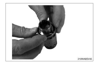
(7) Fit the cross pin (11) into the spool/sleeve.
