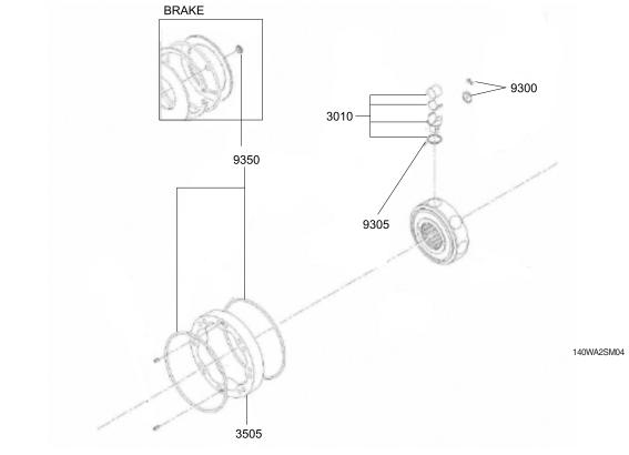
3010 Piston repair kit 3505 Cam 9300 Piston insite kit9305 Piston ring repair kit
