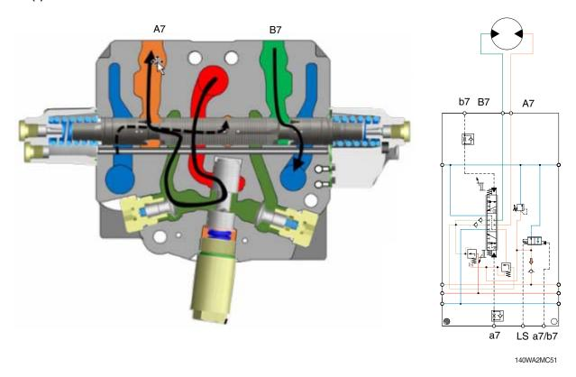
Against LUDV functionality, the LS section is not affected by parallel movements, as long as the system is able to build up the required pump pressure.
