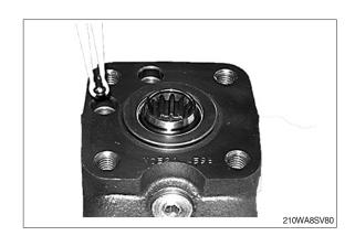
(41) Place springs with trust pads (26) over the two balls.
