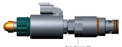
Tool : Spanner 30 Tightening torque : 10.2±1.0 kgf.m (73.8±7.4 lbf.ft)
