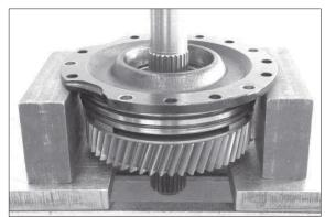
21) Unsnap retaining ring and disassemble ball bearing from cover.
