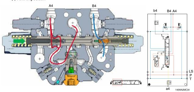
When the pilot pressure is led to the port a4, the oil from the pump flows to the cylinder port A4 and oil from the cylinder flows into the tank through the cylinder port B4.
