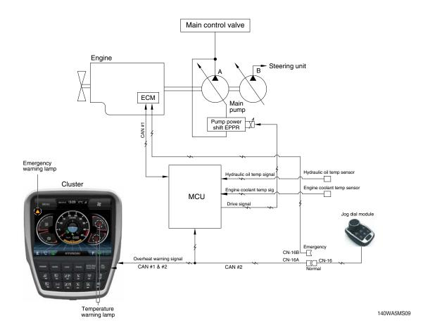
1. If the engine coolant temperature is overheated over 103°C or the hydraulic oil temperature is overheated over 100°C, the warning lamp is ON and the pump input torque or the engine speed is reduced as below logic table.
