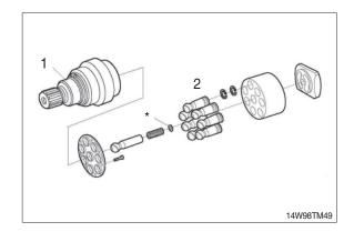
(1) Remove fixing screw (cylinder). Remove cylinder.
