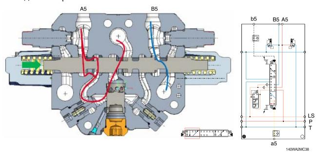
When the pilot pressure is led to the port a5, the oil from the pump flows to the cylinder port A5 and oil from the cylinder flows into the tank through the cylinder port B5.
