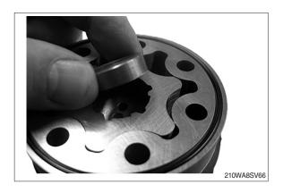
(28) Place and rotate the cardan shaft (51) with the big diameter end until it moves in gear with gear wheel of gear set (17).
