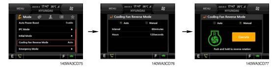
· Manual: Rotate the fan with reverse direction while pressing the button "Excute".
