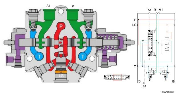
The spool is in neutral position, pump is in low pressure stand-by. The A1 and B1 ports are not connected to the pumps nor the tank.
