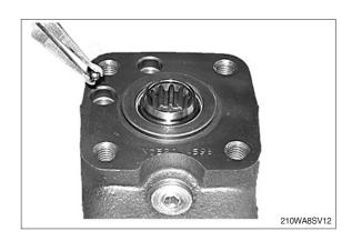
(4) Screw out the seats for shock valves (28). O-ring (41) is fitted on seat (28).
