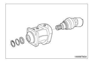
(1) Screw in threaded pin into center pin. Fix the cylinder with disc and locknut. M8  $\times$  105  $\ell$
