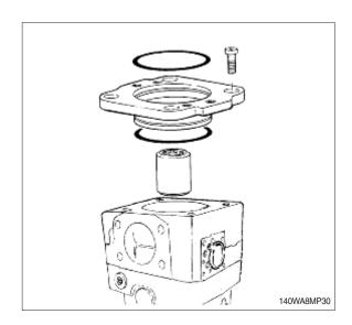
(5) Mark position of the connection plate. Loosen connection plate fixation.
