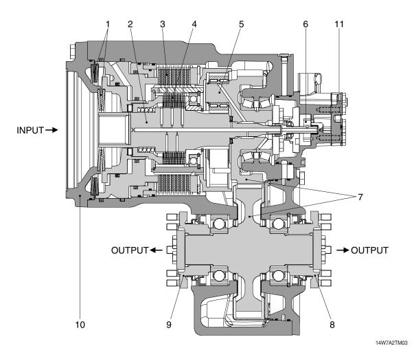
Cup spring Planetary drive 9 Output flange-front axle 1 5 2 Input shaft 6 Lub oil pump Travel motor attachment 10 3 Disk brake 7 Spur gear drive 11 Shift interlock Disk clutch 8 Output flange-rear axle
