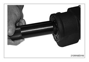
(11) Grease the shaft seal (Roto Glyd, 5) with hydraulic oil and place them on the tool. Ensure that the Roto Glyd seal is placed on the insertion tool as per the photograph.
