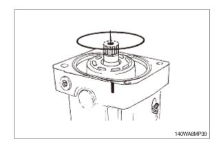
(4) Remove cylinder with pistons.
