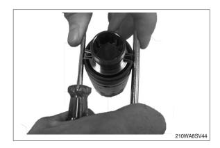
(6) Guide the ring (10) down over the sleeve. The ring should be able to move free of the springs.
