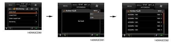
· The active faults of the MCU, ECM, FATC, AAVM (option) can be checked by this menu.
